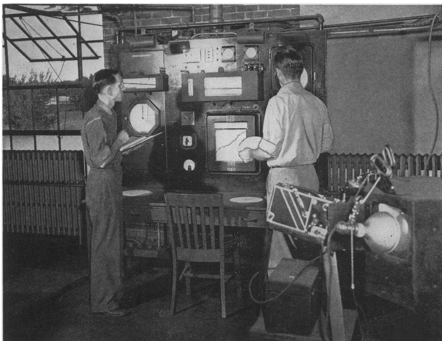
SMOKELESS FURNACE —Scientists of the University of Illinois are checking its efficiency with technical laboratory instruments. With the same amount of coal it gives an estimated 50% more heat than a standard furnace.
