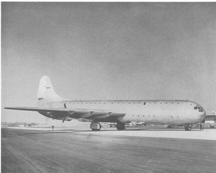
RIVAL —In weight carrying capacity, this new giant transport rivals Hughes' Hercules flying boat. The Consolidated-Vultee XC-99 is the world's largest land-based plane and the Air Force's largest transport capable of carrying 100,000 pounds of cargo.
