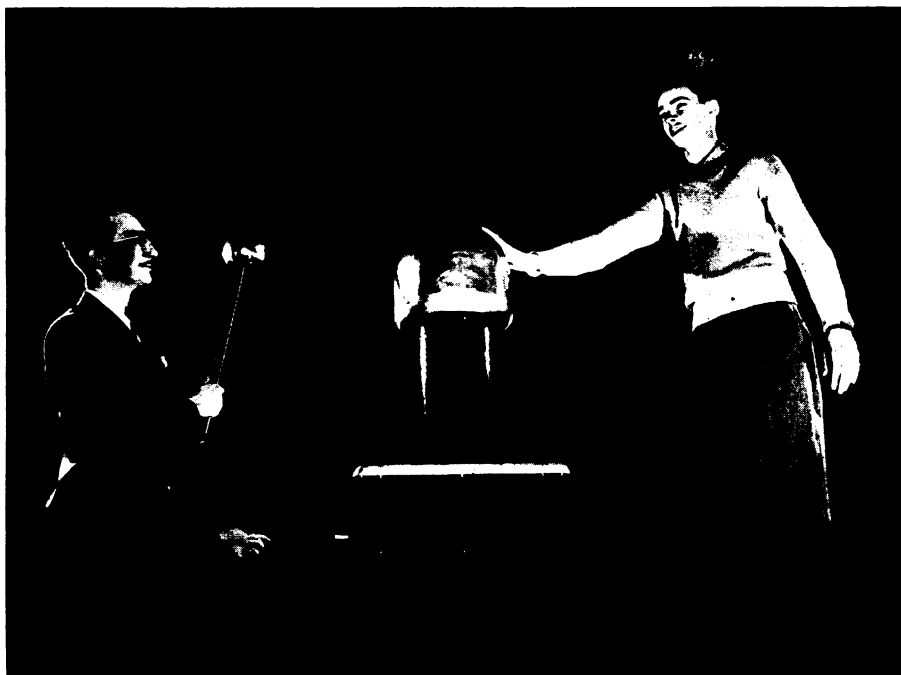
MAKES YOUR HAIR STAND ON END —By touching the dome of this model Van de Graaff electrostatic generator, used in nuclear processes, the young man on the right got a shock of static electricity which made his hair rise vertically. This is one of several scientific instruments being shown at the atomic energy exhibit.
