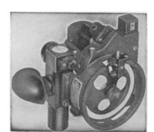
POLARIZING VARIABLE DENSITY ATTACH-MENT FOR BINOCULARS
