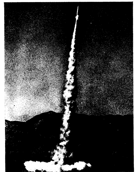
NEW LIQUID-FUELED MISSILE —Shown here leaving the launching rack, the aerobee will be used to carry scientific instruments for upper air exploration.
