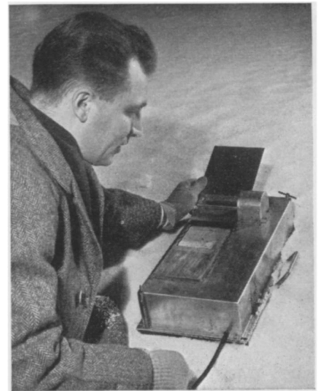
SNOW CRYSTAL RECORDER— This instrument, which prints on paper the geometric shape, size and frequency of occurrence of snow crystals falling in a storm, is shown being observed by one of the men who developed it—Raymond E. Falconer.
