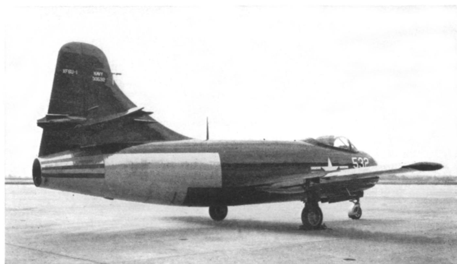
AFTERBURNER —This cylindrical device on the rear will be installed on Navy Pirate fighting planes.
