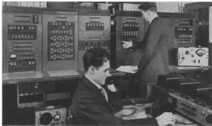
The engineer in the foreground talks over the test circuits which the other engineer sets up on a "circuit simulator."
