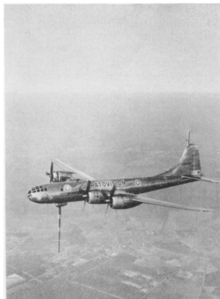
FLYING TELEVISION STATION —This modified B-29 picks up programs from the ground station on the antenna projecting above the tail and re-broadcasts from the long mast-like antenna at the nose of the plane.
