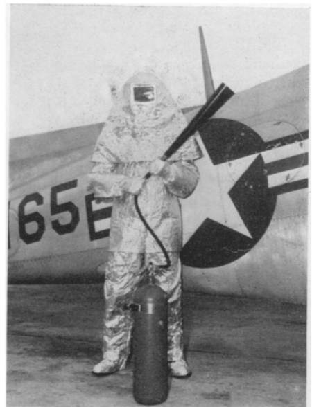
FIRE-FIGHTING SUIT —Made of aluminum foil laminated to a smooth cloth base, tests showed that the wearer could come within two feet of a 1500-degree fire with his body temperature rising only one degree. The suit reflected more than 99% of all heat rays. The helmet window is a one-way mirror reflecting rays directed at it from outside.
