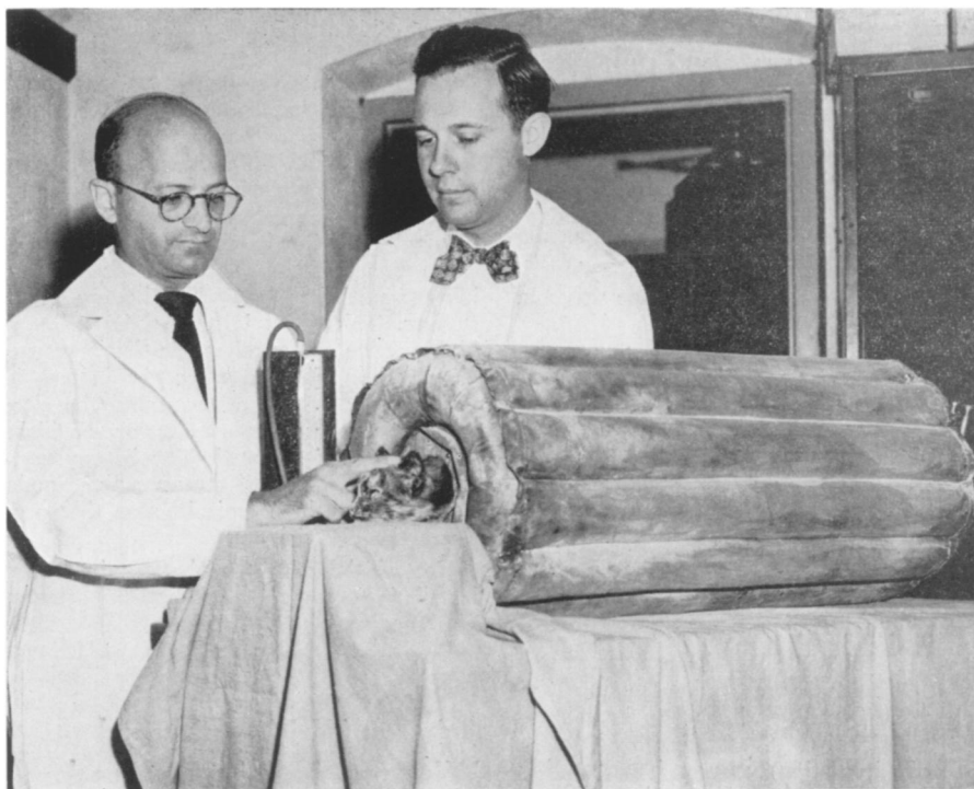
NEW LIGHT-WEIGHT "IRON LUNG" —This cat is breathing artificially in the new Yale cloth respirator. It was developed by Dr. Harold Lamport, left, and Dr. Ralph D. Eichhorn, right.
