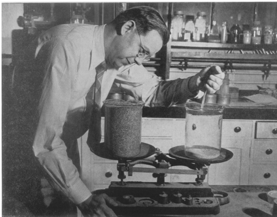
EXPANDED MINERAL —Featherweight vermiculite, excellent for roofing or insulation, weighs only about a tenth as much as sand, being measured at right.
