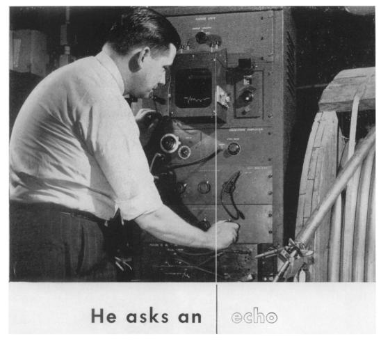
Radar sends out pulses of electric waves which, reflected from a target, return to reveal the target's location
