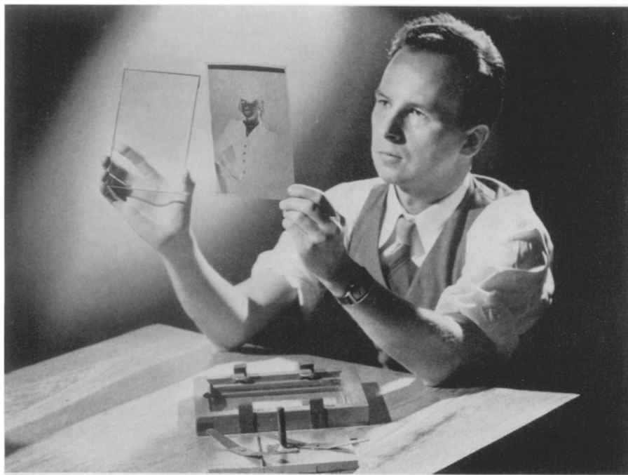
PHOTOGRAPHS PRINTED IN GLASS —This is done by a new process that uses an ordinary negative and ultraviolet light, then heat, to create a positive permanent picture. Dr. Donald S. Stookey of Corning Glass Works is shown examining a negative and a piece of photosensitive glass before he inserts them into the printing frame on the table.
