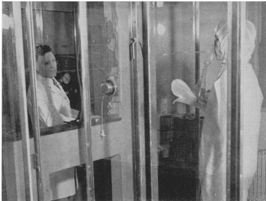
SMELL-PROOF ROOM —Testing for odors, Dr John V. Haralson of Cornell University sniffs an isolated odor from an "olfactory stimulator" while the long glass tube carries off his exhaled breath. The fiberglas envelope in which he is garbed and the equipment in the chamber were designed by Dean Foster, at left.
