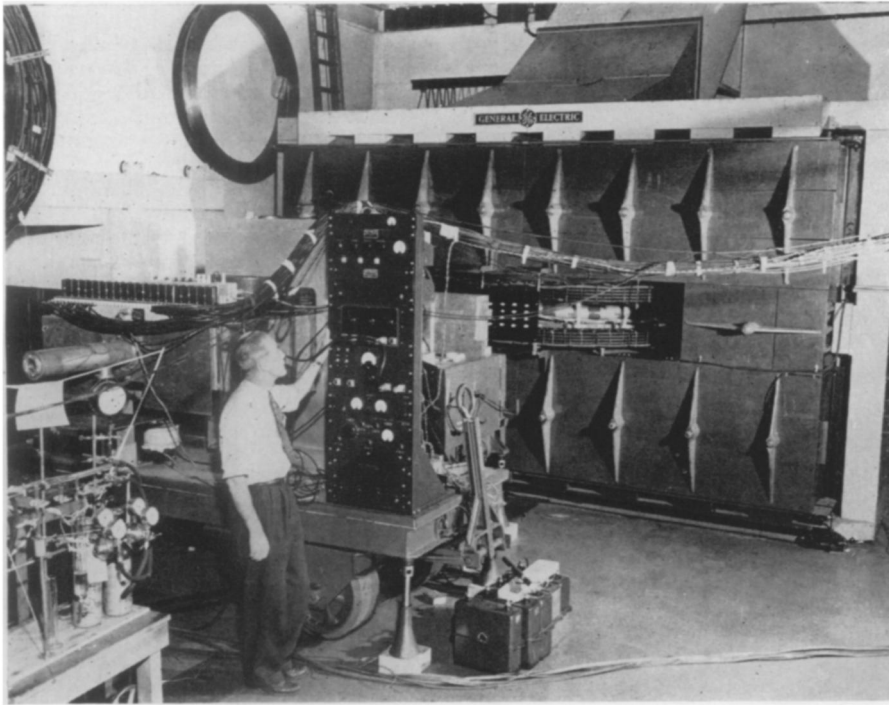
DETERMINES ENERGY DISTRIBUTION —Shown in place before the 100,000,000-volt betatron in the General Electric Research Laboratory is the gamma ray spectrum analyzer used in studying the radiation from this device. It was developed by Dr. James L. Lawson of G-E as a labor-saving device.
