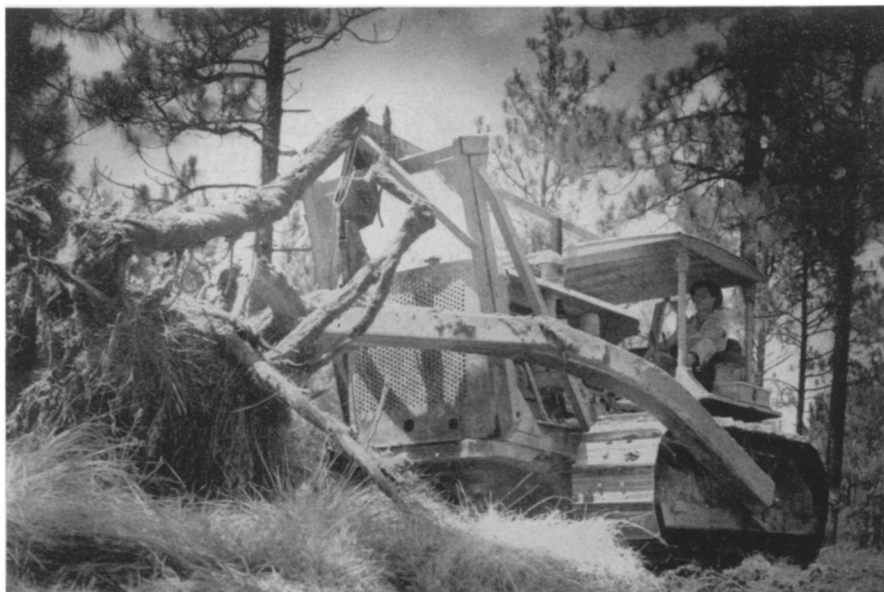
GRUBBING —Uprooting pine stumps is the first step in the manufacture of naval stores products.
