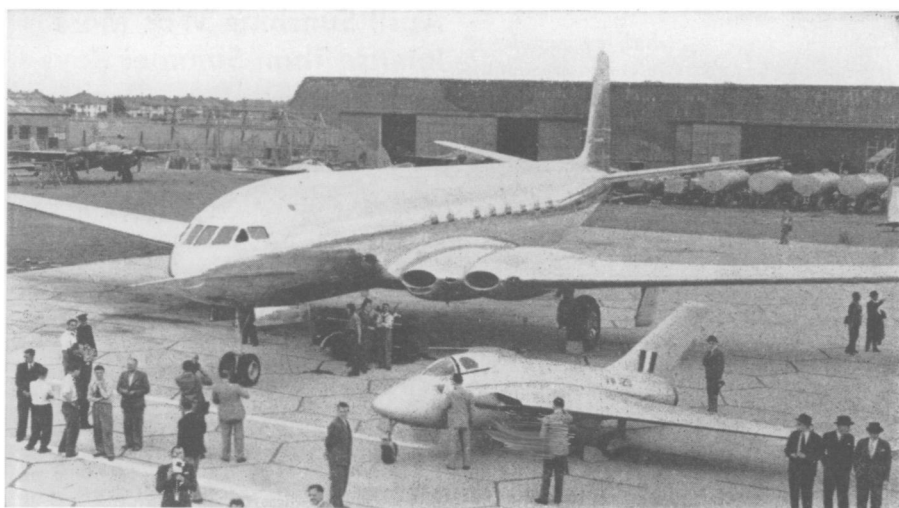
WORLD'S FASTEST AIRLINER —This is Britain's four-engine all-jet airliner, the de Havilland "Comet." It is a low-wing monoplane with a moderate swept-back wing and is expected to have a cruising speed of 500 miles per hour at 40,000 feet. The small jet in the foreground was used to determine wing resistance, stress and strain for the new airliner.
