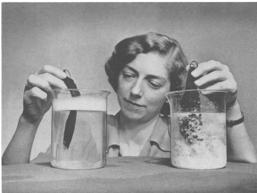
ADVANTAGE OF SYNTHETIC DETERGENTS —Soapless soaps in the left beaker give plenty of suds, even in hard water, while soap forms gummy curds in the right beaker.
