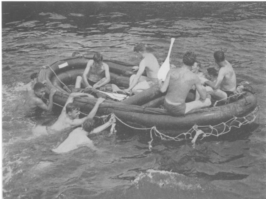
EMERGENCY RUBBER LIFEBOAT —Thirteen men can hold onto the lifelines alongside this boat while there is room for 12 men inside the boat. A Coast Guardsman is preparing to inflate the two six-foot square floor sections which can be thrown into the water to support an additional 10 men.
