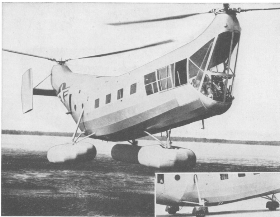
HELICOPTER GETS FLOATING FEET —Nylon floats have been attached to the wheels of this tandem rotored Piasecki HRP-1 "Rescuer" helicopter of the U. S. Coast Guard. It enables it to set down easily on the water for emergency rescues. It was designed by Cmdr. Frank A. Erickson, head of the Rotary Wing Development Unit at Elizabeth City, N. C. The pilot needs only pull a cord to release the floats. Insert photo shows how compactly the floats fold around the landing wheels.
