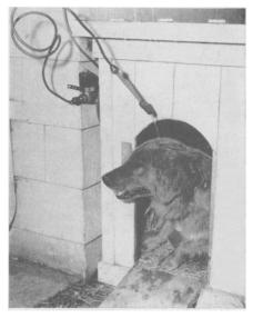
BARK CONTROLLER, for the dog with an early-morning habit of yapping for release from the doghouse, is a homemade apparatus with a microphone for an activator. The microphone picks up the "bark" and starts the mechanism that delivers a squirt of water on the dog's head, as shown in the picture.
