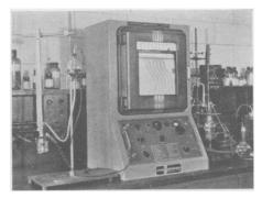
Designed for rapid, accurate polarographic analysis, the new L&N Type E Electro-Chemograph features one piece console design incorporating a built in Speedomax Recorder. The instrument automatically plots diffusion current as a function of voltage and is convenient for both research and industrial process control laboratories.
