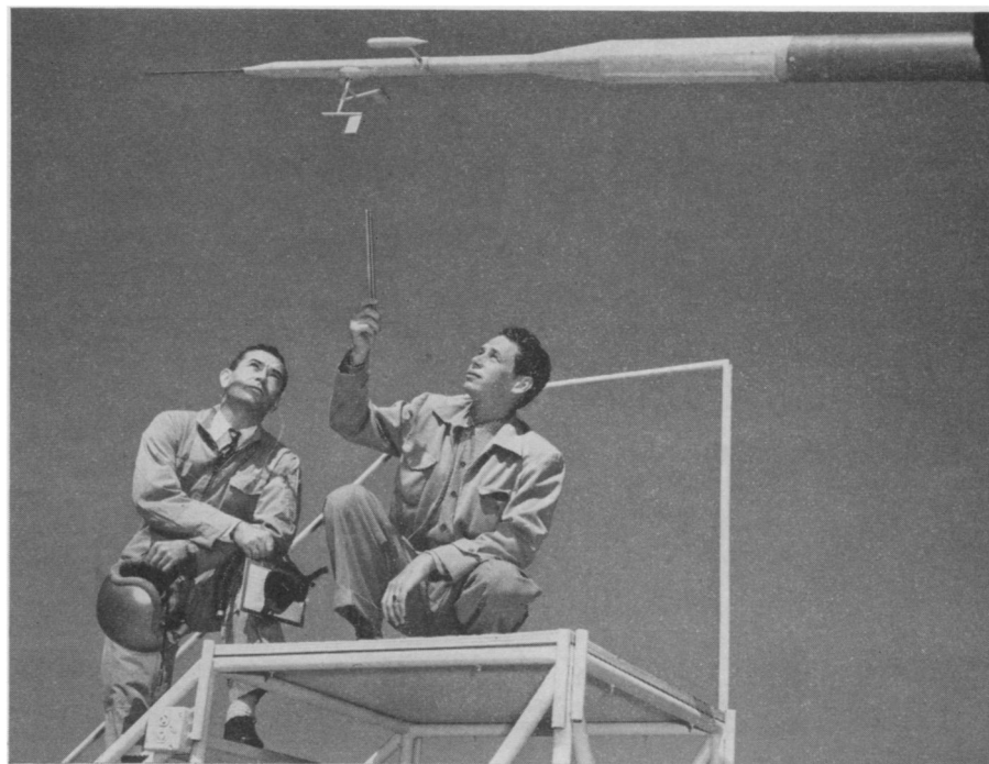
INSTRUMENT MAST FOR FLIGHT DATA —This needle-nosed "spear" probes the atmosphere ahead of high-speed research planes to give instant telemetered readings of air speed, yaw, angle of attack and temperature. It was developed by G. M. Giannini & Co., for Northrop Aircraft, Inc., and is undergoing tests now, being the first all-electric instrument mast to be designed for this use.
