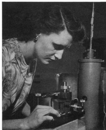
X-RAY MICROSCOPE —Miss Charlys M. Lucht, of the General Electric Research Laboratory, demonstrates an experimental X-ray microscope. The microscope makes it possible to examine directly minute details of internal structure in materials through which light cannot pass.
