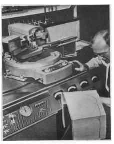
"X-RAY SPECTROGONIO-METER"—Dr. David Harker of the General Electric Research Laboratory studies a record of an unknown chemical sample, drawn automatically by the machine on which his hand rests. The machine makes it possible to determine in a few minutes the chemical content and arrangement of atoms in a chemical sample.
