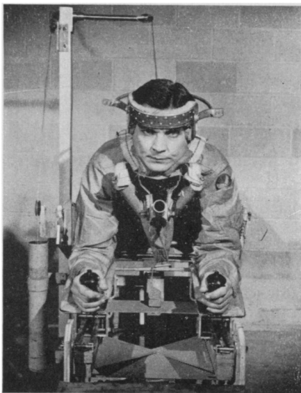
PILOT BED—H. T. Hertzberg, chief of the Anthropometric Unit, demonstrates the prone position pilot bed which eliminates flying fatigue common with the ordinary sitting position and increases tolerance of pilots to gravitational pull.
