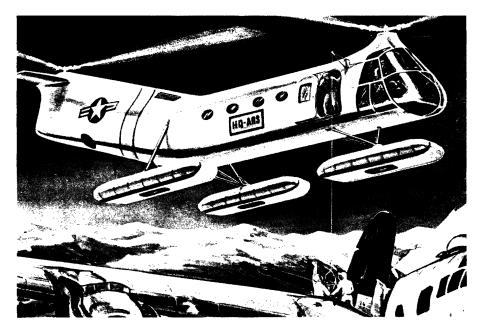
"OMNIPHIBIOUS HELICOPTER"—The world's first helicopter designed specifically for large scale rescue work in the Arctic will be able to land on snow, ice, water, tundra, marsh or land without changing gear. The 20-foot long cabin can accommodate up to 12 litters plus two seats for medical attendants, or 20 troop seats, or as many as 27 persons can be carried in the floor of the big cabin.
