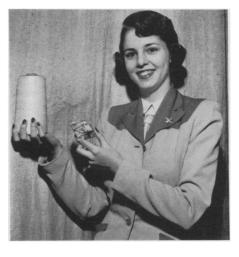
spool of glass fiber in one hand and a sample of mineral asbestos in the other. The fabric is composed of glass yarns interwoven with asbestos yarns.
