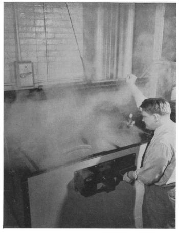
Only an engineer would think of a practical use for this gadget. Faced with the problem of what will happen to street lighting units where smog shrouds a city, this "box" becomes a vital piece of testing equipment. For, with it, the effects of 20 years of corrosion exposure can be determined in 1,000 hours.
