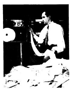
"SMOKE PUFFS" RECORDED— Prof. L. A. Manning of the Stanford Electrical Engineering Department examines a paper tape recording of the drift of meteoric "smoke puffs" detected by radio equipment. The drift gives clues to the speed and direction of upper atmosphere winds.
