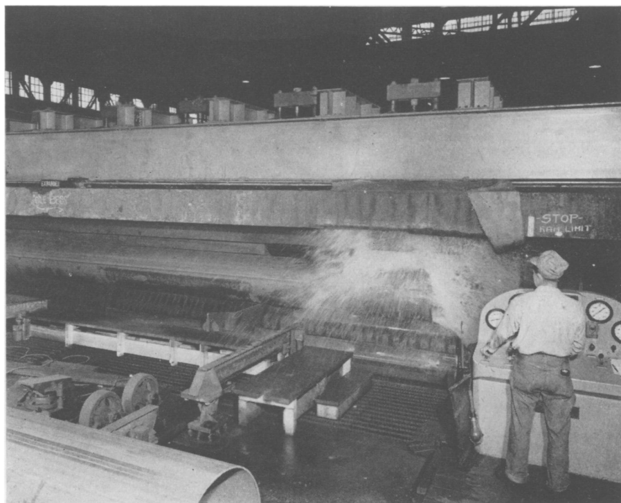
PIPE STRETCHED —Water gushes forth after stretching diameter of steel pipe. Pressure is reduced before the ram is withdrawn from the unusual machine which uses the power of water under pressure to stretch the diameter of heavy pipe as much as one-half inch.
