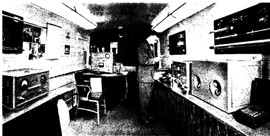
FOR ATOMIC BOMB DEFENSE —All the instruments needed to detect and measure radioactivity are mounted in this truck-carried laboratory. In case of explosion, this mobile laboratory could speed to the scene to test for radiation, identify type of rays, and measure danger. It is built by Radiation Counter Laboratories, Inc., of Chicago.
