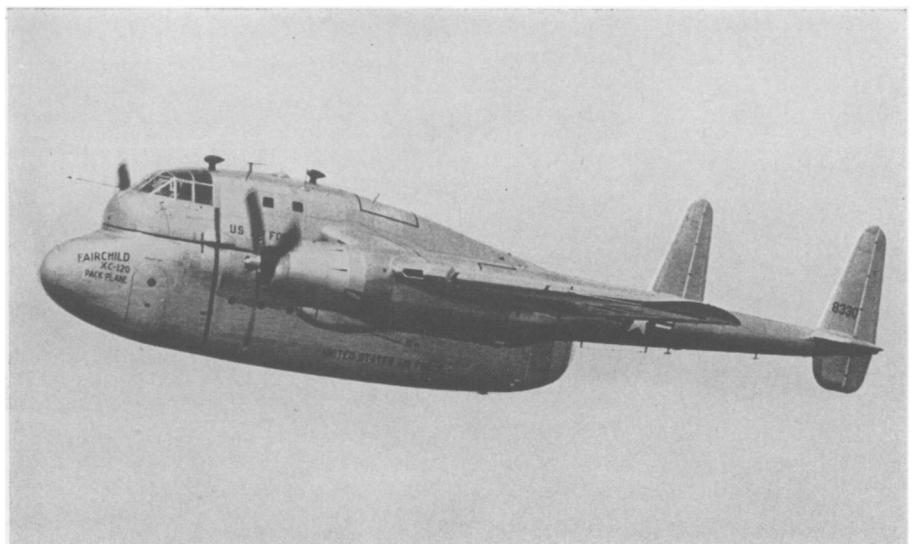
FIRST DETACHABLE FUSELAGE —The giant detachable cargo compartment in a military transport allows for faster ground handling and loading times. The compartment can also be fitted out as a surgical operating room or a forward photographic laboratory for advanced areas.
