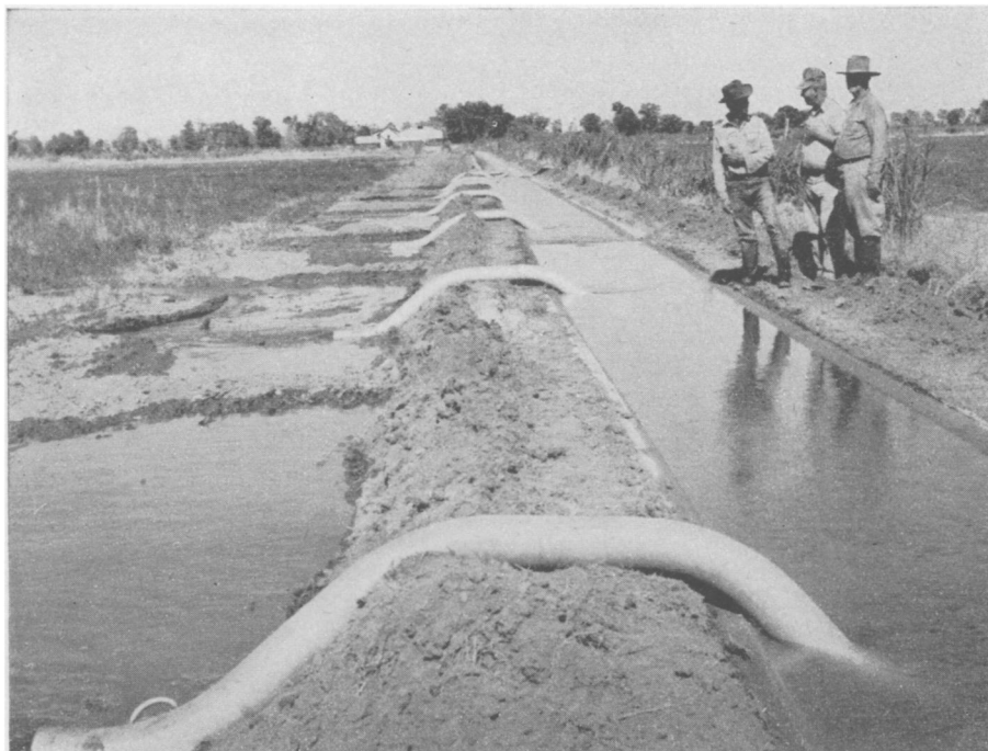
KINGSIPHON —The giant aluminum siphon for ditch and flood type irrigation systems delivers approximately 320 gallons per minute with a 6-inch head. Rated 62% efficient, this siphon is easy to handle as it weighs only 13 pounds.
