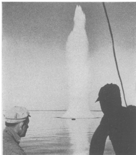
ON THE SEA —A geyser of water shoots 100 feet into the air as the suspended charge is detonated, sending shock waves to be picked up by the string of seismometers along the shot line.
