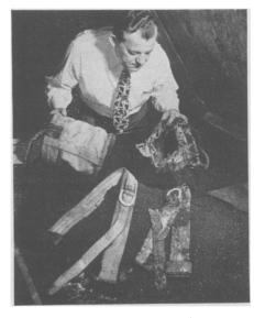
MILDEW CONTROL—The canvas bucket and webbing at the left have been protected against mold decay by one of the Cunilates developed for the Air Force. Victor N. Kalberg, who developed solubilizing technique, compares them with similar items which almost completely disintegrated after 28-day soil burial test. The Cunilates are available in permanent and non-toxic solutions and emulsion.
