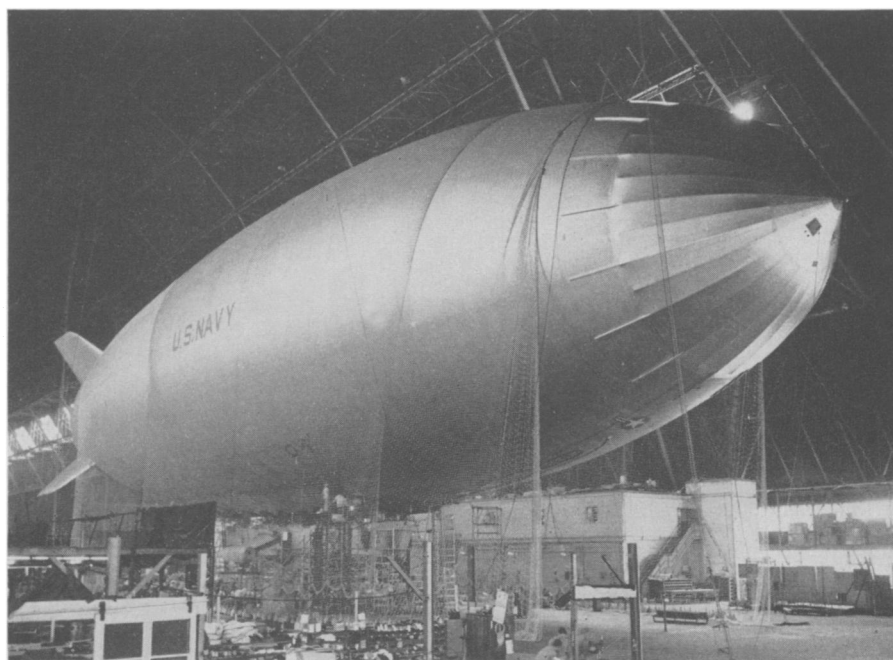
ANTI-SUBS —The ZPN airship, newly developed for the U. S. Navy, will help to combat the submarine menace in the event of future war. The net, shrouding the huge ship, is used to hold the helium-filled envelope down while the control car and other fixtures are being attached.
