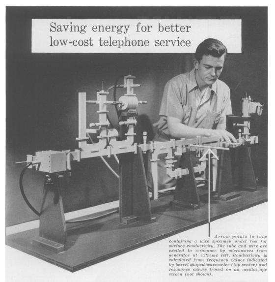
In the waveguides which conduct microwaves to and from the antennas of radio relay systems, current is concentrated in a surface layer less than 1/10,000 inch thick, on the inner surface of the waveguide. When these surfaces conduct poorly, energy is lost.
