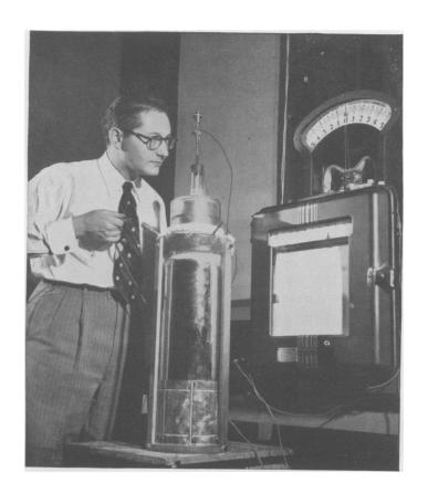
When temperatures drop low enough...say 450 degrees below zero... bouncing molecules come to a virtual standstill, eliminating resistance to the flow of electricity so that current will flow indefinitely—even after the power supply has been cut off.
