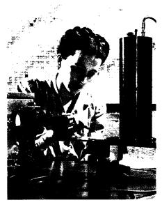
IDENTIFIES BIG THREE—The universal scintillation counter analyzes the white square of paper which contains the smear from object suspected to be contaminated. The instrument is able to check the smear for presence of alpha, beta or gamma rays, which are the "big three" of nuclear radiation. Mrs. Ethelyn Langdon, engineering assistant, operates
