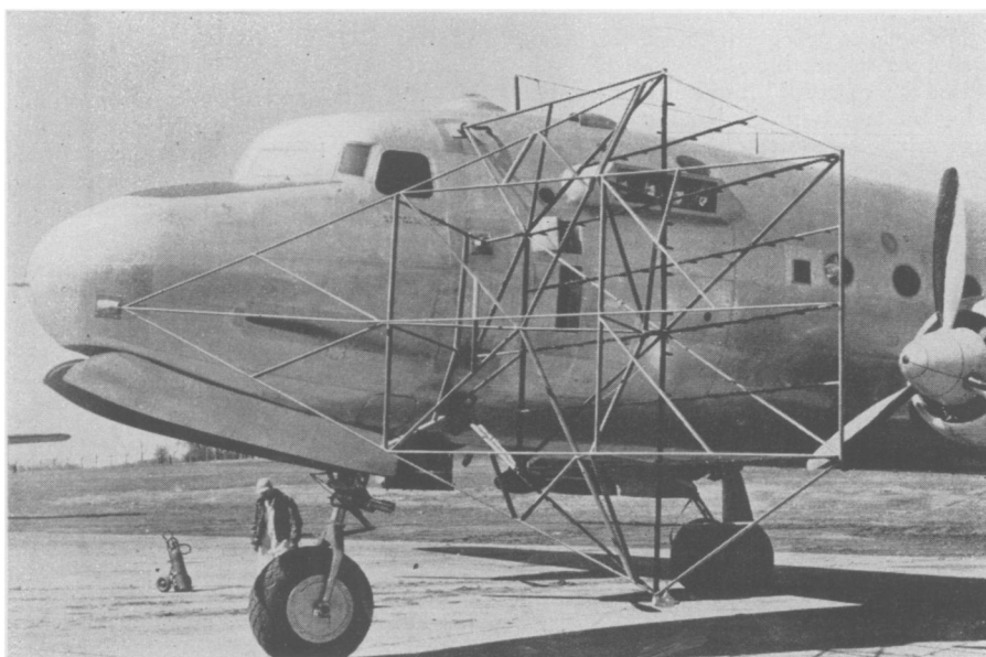
"SQUIRTING GERTIE" —"Gertie" is doing her bit by helping engineers fight the dangers of aircraft icing with experiments at Ypsilanti, Mich. The plane carries outside an elaborate maze of aerodynamically fitted pipes containing nozzles which can turn ordinary water into rain, snow, fog or mist. It creates only a minimum of drag, slowing down the plane to which it is attached by less than 10 miles per hour.
