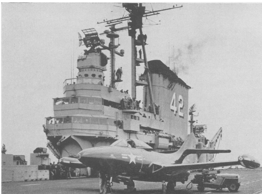
TRICYCLE JEEP —The tricycle-gearred jeep is nimble as a cat, turning in a circle which has a 7-foot radius. Used to energize jet aircraft and military planes, it is also valuable for towing disabled planes out of the line of flight traffic.
