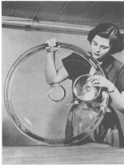
The 26-inch blank in the picture is contrasted with a 6-inch reflector.
