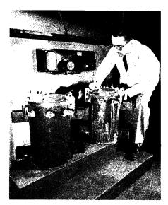
PAINT SANDWICH—Still bright and shiny after 1,000 hours of continuous exposure to corrosive salt water spray is the distribution transformer tank at left, which is coated with a new three-decker paint. The tank at right, coated with a standard finish, quickly fell victim to the salt water attack.
