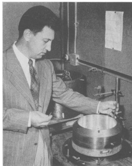
MEASURES LIGHT SPEED—Dr. Edward Ginzton is showing the cylinder used in Stanford University experiments to obtain a more accurate measurement of the speed of light.
