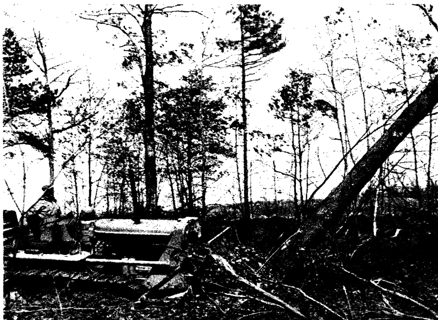
LIGHT BUT STRONG —This airborne bulldozer is light enough to be flown to advanced combat positions, but is capable of doing the heavy work of its weighty predecessors.
