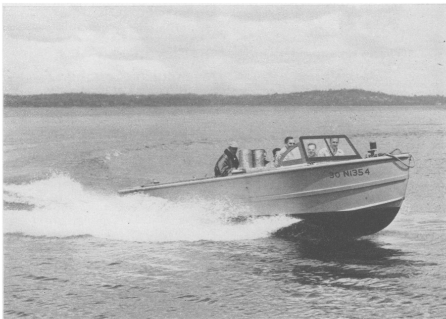
TESTING GAS TURBINE —This 24-foot Navy personnel boat is pictured making a test run of the Boeing gas turbine engine which the Navy plans to use to power minesweepers.
