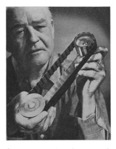
SPOWER transmission belt with teeth, shown in the picture, is made of rubber and fabric and is designed to replace flat belts, V-belts, chain drives and gears in hundreds of applications. This noiseless, non-slip belt makes possible higher operating speeds than other drive mechanisms.
