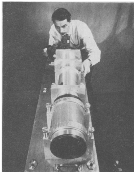
"CLOSE-UP LENS" —This special lens assembly, designed and built by Kurt Kriegsmann of the Naval Ordnance Laboratory, enables a photographer to take a close-up picture of objects over much longer distances than previously.
