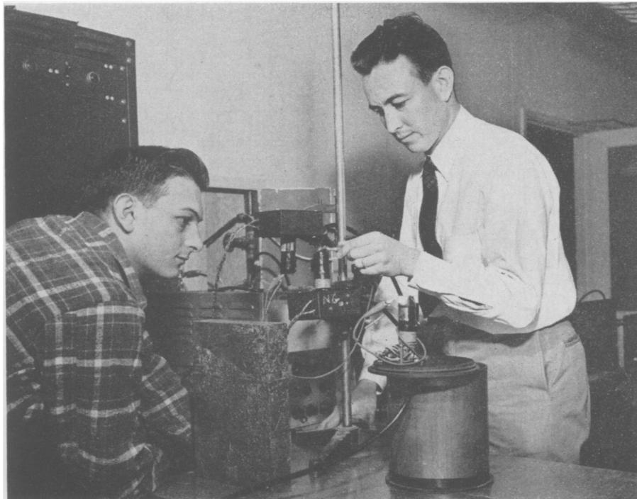
FAST MEASUREMENT —Norman Shiren, research assistant, and Dr. Richard F. Post, adjust photo-multiplier tube used in Stanford experiments which have counted an atomic particle in a billionth of a second.
