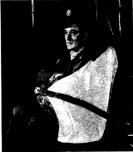
NET HARNESS —This safety harness is designed to protect airmen from crash impact and from take-off and landing jolts.
